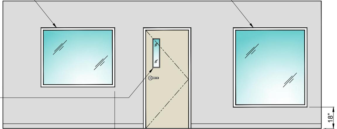
RAY-BAR X-RAY SAFETY GLASS OR FIRE RATED GLASS IS PERMANENTLY LABELED AS MEETING ANSI Z97.1 AND CPSC 16 CFR PART 1201 CAT 2 AS REQUIRED BY IBC 2406 FOR IMPACT RESISTANCE.
